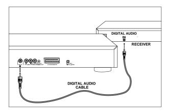
For multichannel sound, your player provides both digital and analog audio outputs.
